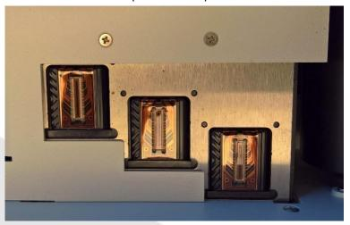
For this purpose, the print heads can be removed and re-inserted. Please also refer to Chapter 10.8 Inserting / replacing print heads.
